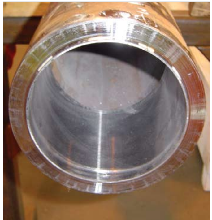
J-bevel and counterbore weld preparation for SCR fabrication
